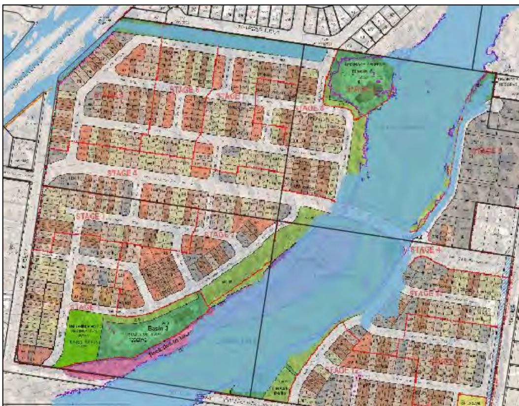
Figure 3.9 1:100 AEP Flood Height – IG24 Waterway Crossing Extreme Blockage Sensitivity (Scenario 2)
