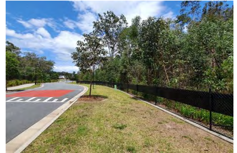
Figure 4.2.8. (photo D de Villiers) Reduced fencing height creates a partial barrier to koalas and discourages koalas climbing the fence and entering the road corridor.
